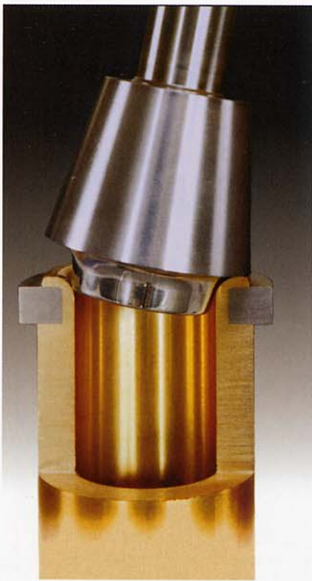
Cross-section of tubular end of one part flared over by orbital forming tool to capture a ring securely.
