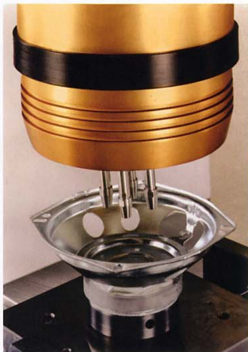
This multipoint orbital unit flares out four semipierced posts simultaneously to secure a speaker basket stamping to the magnet without damaging the brittle magnetic material.
