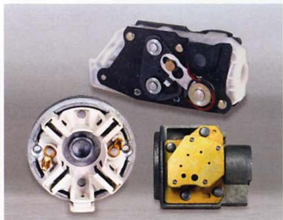
Typical parts assembled without the use of loose fasteners. Integral diecast studs, pins, tabs or bosses are flared or headed by orbital forming to secure mating parts.
